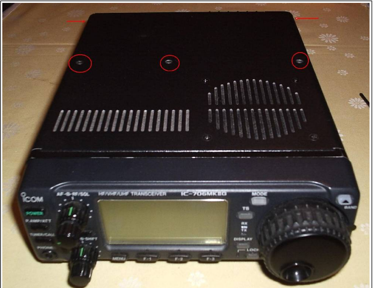
Remove three screws from the upper panel and two on the side as shown.
