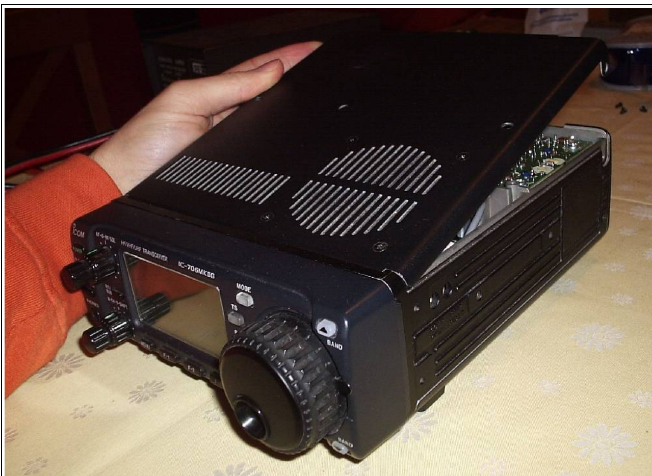
Carefully lift the top cover as shown, starting from the back of the radio.
