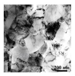
Transmission electron microscopy micrograph of nanostructured copper prepared by powder metallurgy.
