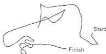
Figure 2-2. Scratch left on the floor by a kitchen range in the 1933 Long Beach California earthquake. [Reprinted in redrawn form, by permission of Princeton University Press, from Nicholas Hunter Heck, Earthquakes (Princeton, New Jersey: Princeton University Press, 1936, 1964), Original drawing by W. L. Luxton.]
